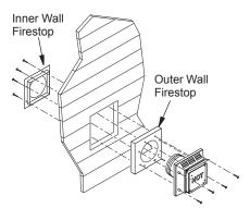
Figure 13 - Installing Outer Wall Firestop (Combustible Exterior Wall)
